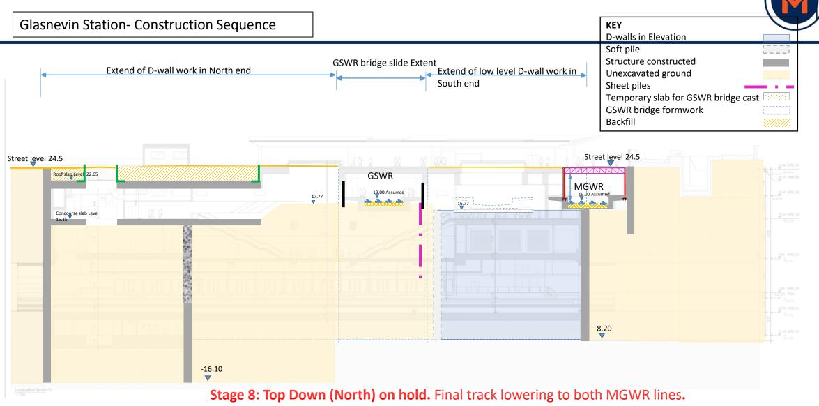
Commence GSWR bridge deck construction and prep works for Bridge Slide. Install formwork on Temporary slab
